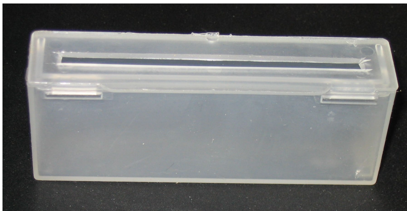
Microscope Slide Mailing Container Modified to be an Extraction Chamber.
